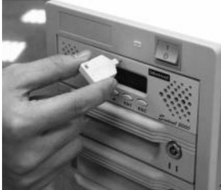
Use the bezel included in the package to remove front panel module.
