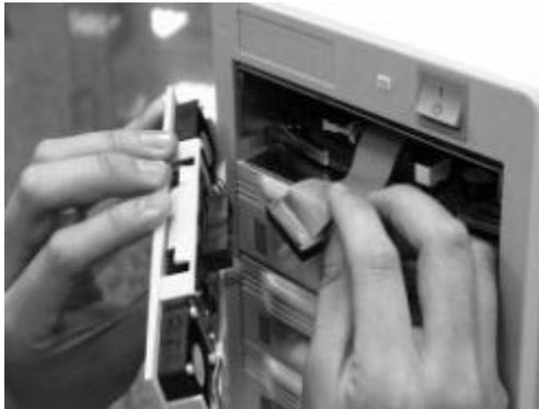
Unplug the ribbon cable which connects between the front panel module and the controller main board.
