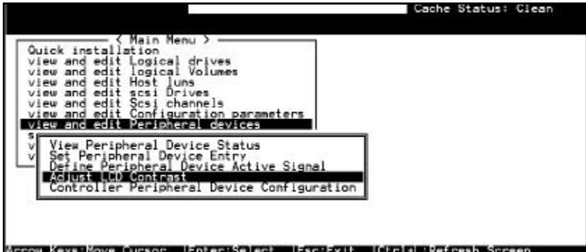
Select “View and Edit Peripheral Devices” from the main menu, press **[ENTER]** to confirm. Select “Adjust LCD Contrast,” and then press **[ENTER]**.
