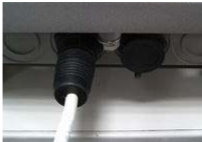
Figure 16 - MIL-C-5015 Style Ethernet Connector
