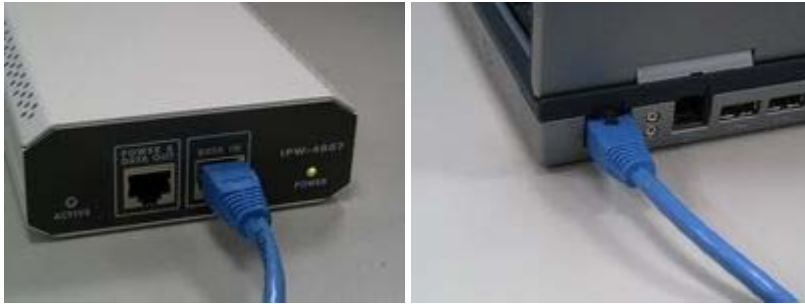
Figure 15 - Ethernet Cable With Inline power injector
