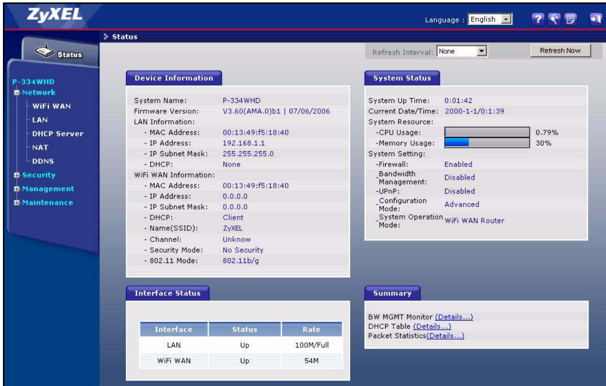
Figure 10 Web Configurator Status Screen (WiFi WAN Router Mode)
