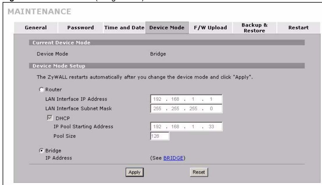
Figure 191 Device Mode (Bridge Mode)
